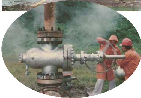
Bleed/Side Valve-Through Conduit type Expanding Gate Valve
