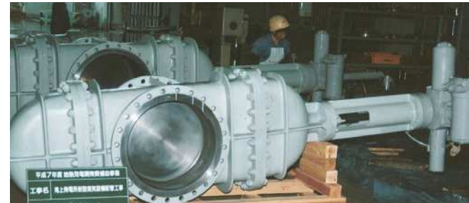
Through Conduit type Expanding Gate Valve for piping line
