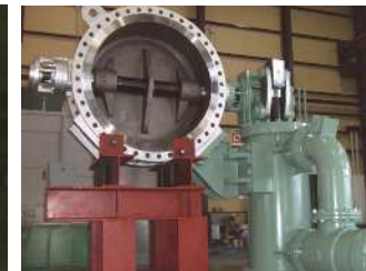
Main Stop Valve for Turbine (Butterfly Type)
