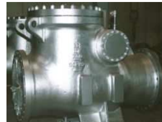
Main Stop Valve for Turbine (Swing Check Type)
