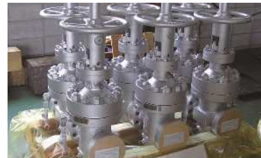
Bleed/Side Valve-Through Conduit type Expanding Gate Valve
