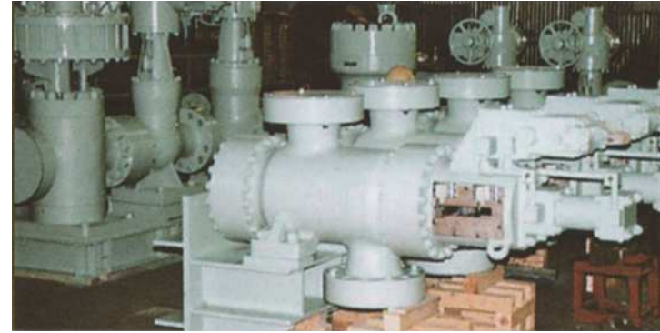
Various Valve for Descaling System
